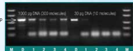
DreamTaq™ DNA Polymerase outperforms conventional Taq DNA Polymerases from different vendors in amplification of different amounts of human genomic DNA M - FastRuler™ Low Range DNA Ladder, ready-to-use (#SM1103) D - DreamTaq™ DNA Polymerase (#EP0701) 1-4 - Taq DNA polymerases from different vendors
