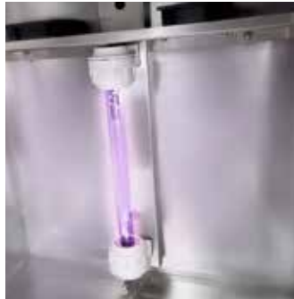
Air UV recirculation system in the chamber
